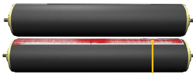
Pressure film records nip impression
