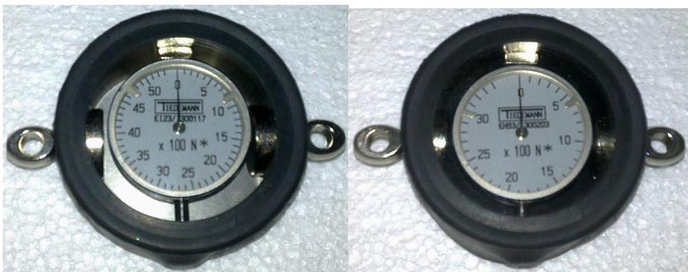
Dynamometer for Y-Cable Tensioning Device with up to 5 kN and 3.5 kN
